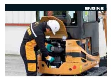
The new 11.3 kW Mitsubishi engine provides plenty of power for the series 2 machines. Centralised access, with all service points easily reached from beneath the engine canopy, reduces maintenance time and cuts service costs. The battery can be accessed from beneath the bonnet when necessary, further reducing downtime. All liquid checks can be carried out from ground level for maximum operator safety and rapid start-up each day.
