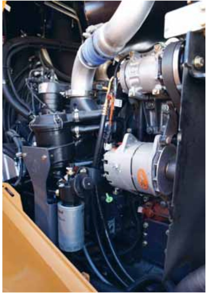
Fuel filter and engine oil service points are easily accessible from the left side while the other filters are behind the right stairs
