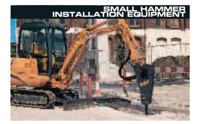
CASE installation accessory options have been designed to allow multi-carrier breaker applications, supported by CASE Operator and Parts Manuals. The breaker can be fitted without modification to all CASE machines. This is an attractive feature for the Rental Industry.
