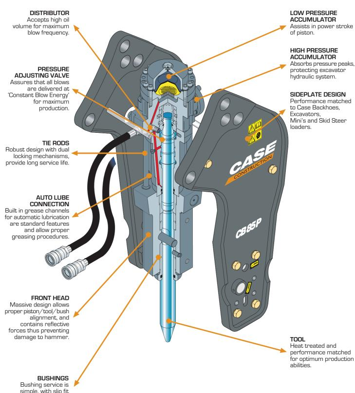
Busning service is simple, with slip fit design for easy removal and replacement, and includes a 'field replaceable' lower bushing.
